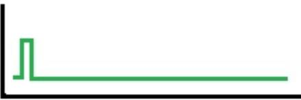
**Green fast flashing light** indicates that diffusion has successfully completed. Panel indicates **"Pulverizing OK"**
